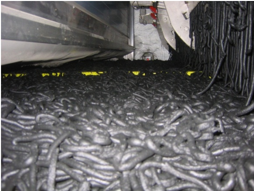
Dewatered sludge "spaghettis" from Evaporis LT™ (Low Temperature Thermal Drying)
