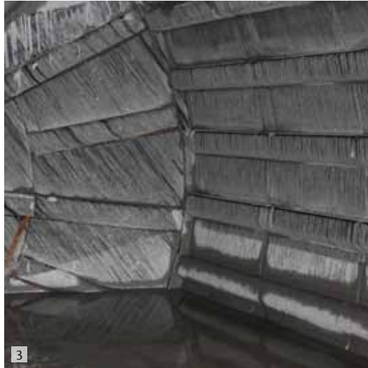
3. Patented Vulco® heavy-duty metal cap shell plate for extended service life in large diameter AG, SAG and ball mills
