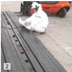
1. Typical grate discharge assembly 2. New composite SFL plates for SAG mill application
