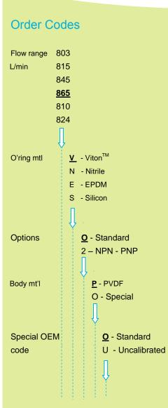
e.g. <u>865-VOP-O</u> is a flow range of 0.25 to 6.5 L/Min, Viton<sup>TM</sup> seal, standard, PVDF bodied flowmeter with a 6 point traceable water calibration.
