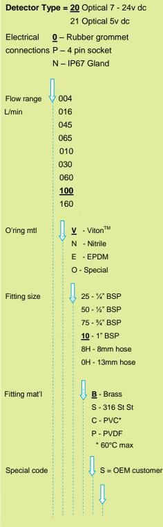
Order code example: -  $\underline{220-100-V-10-B}$  is a flowmeter with a flow range of 4.0 to 100 L/Min, Viton<sup>TM</sup> seal and 1" BSP brass fittings with a standard 6 point traceable water calibration.
