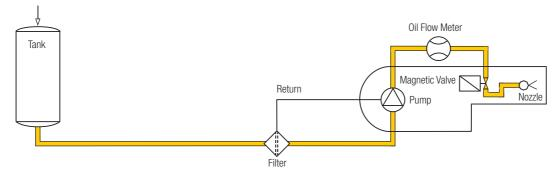
Mounting on suction side of pump (burners)
