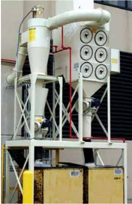
DFT/CYCLONE on Paper Processing 5,300 cfm (9,003 m 3 /h)
