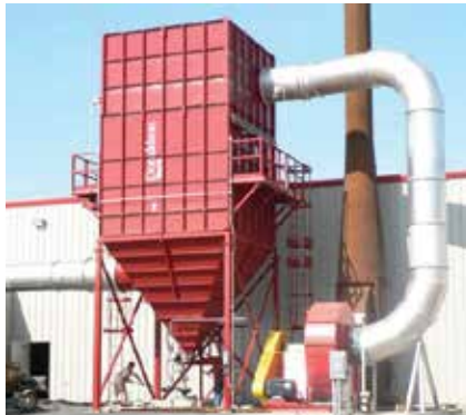
MB on Glass Processing 25,000 cfm (42,466 m 3 /h)
