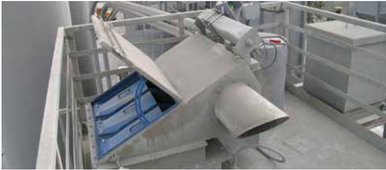
CPV - Pneumatically Filled Storage Bin 1,200 cfm (2,038 m 3 /h)
