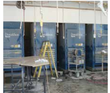
DWS on Granite Finishing 22,000 cfm (37,370 m 3 /h)
