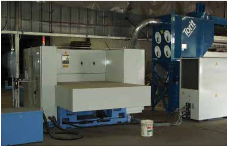
DFO on Laser Cutting 3,100 cfm (5,266 m 3 /h)
