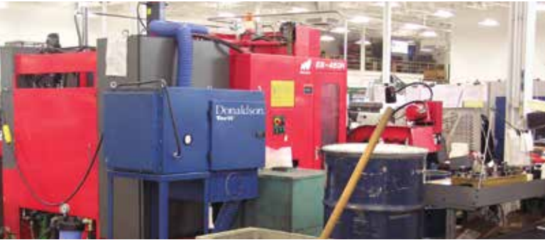
DMC on Machining 800 cfm (1,359 m³/h)
