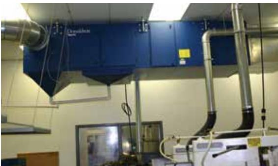
MODULAR MEDIAFILTER™ on Grinding 2,000 cfm (3,397 m³/h)
