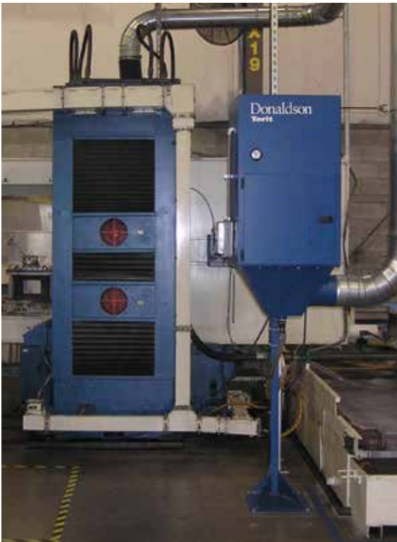
WSO - Horizontal Grinder 850 cfm (1,444 m³/h)
