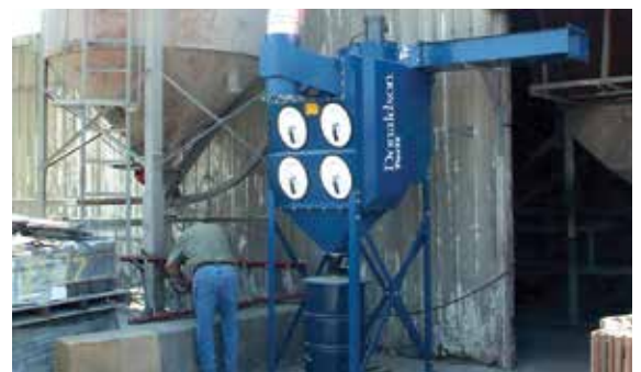
DFO - Concrete Roof Manufacturer 3,000 cfm (5,096 m 3 /h)
