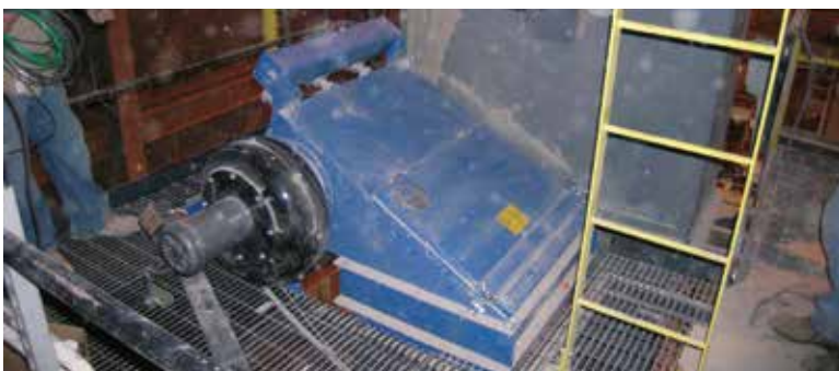
CPV - Bucket Elevator 1,200 cfm (2,038 m 3 /h)
