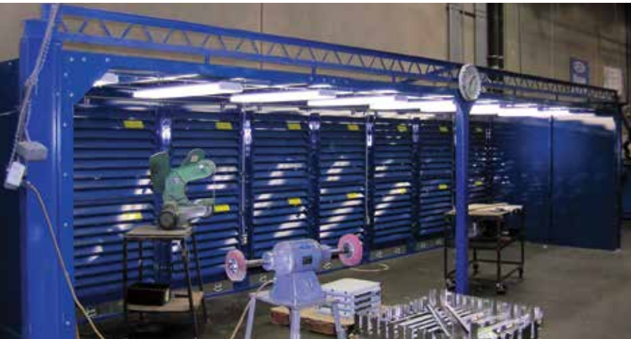
DWS ON Custom Hand Grinding 38,500 cfm (65,398 m³/h)
