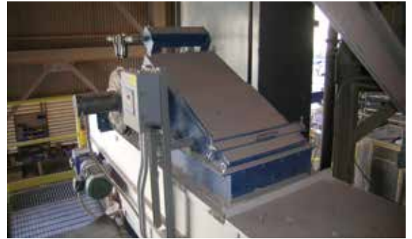
CPV - Weigh Belt Feeder 800 cfm (1,359 m 3 /h)
