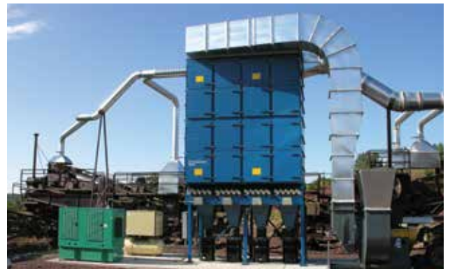
DLMC on Rock Crushing 41,000 cfm (69,645 m 3 /h)
