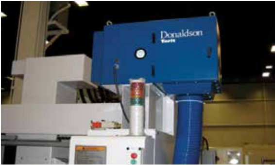
DMC on Wet Machining 390 cfm (662 m³/h)
