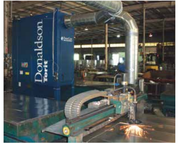
TG on Plasma Cutting 3,400 cfm (5,775 m 3 /h)
