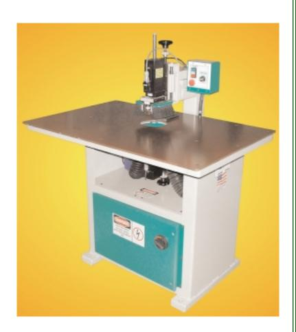
Upper and lower 0.7HP, 12,000 RPM motors with potentiometer control for inverter drive. Pneumatic cylinder with foot pedal control for raising and lowering of upper trimming unit.
