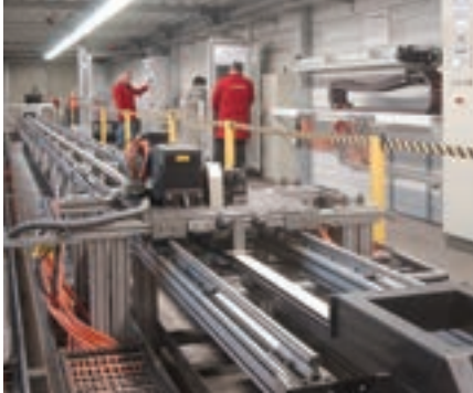
Drag chain test system
