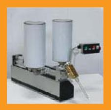
Metering, mixing and dispensing machines are useful for the automation and control of higher volume two-part systems. For the most part, these machines
