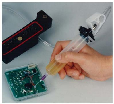
*Figure 1 – Simple pneumatic dispensing*
