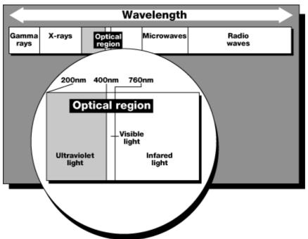
Figure 2 – The Optical Region of the Electromagnetic Spectrum
