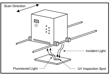
Figure 4 - On-Line Optical Inspection Scanner
