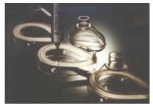
Figure 6 – Face Mask Bonded with Light Cure Adhesive
