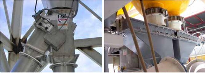
Vortex fabricated transitions are available in aluminium, carbon steel and stainless steel. Fabricated Transitions provide flexibility for customers when installing our valves with existing equipment. Transitions can address custom flange to flange dimensions. They may also be fabricated to contain flanges that match special bolt patterns, tube stubs with or without sock beads, or blind flanges that allow “in the field” hole placement and installation.
