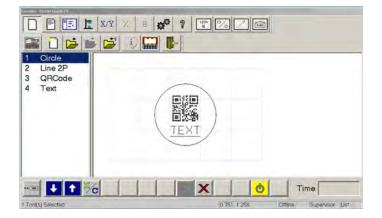
be imported for marking. Non-printable fields can be created to clearly display a graphical representation of the part being marked. Commands may be defined to perform specific tasks during the marking cycle (e.g., Pause, Go to, Input, or Output).
