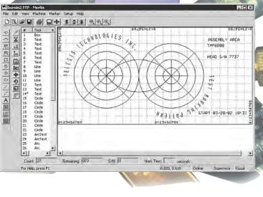
Marking "tools" available include text (at any angle), arc text, rectangles, circles, ellipses and lines. Multiple fields can be grouped and saved as a block to form a logo, or import logos via DXF CAD files.
