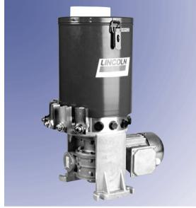
The 215 centralized lubrication pump is a highpressure multi-line pump that can drive up to 15 adjustable pump elements and is used in progressive automated lubrication systems. It is capable of handling direct supply of lubrication points or as a central lubrication pump in large sized progressive systems.
